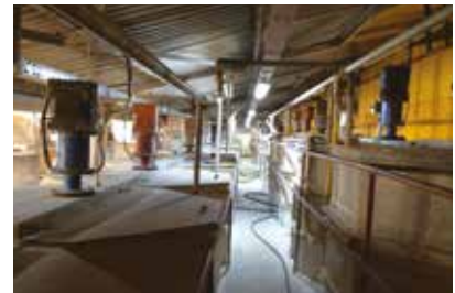
Glazur Mixer - 185 Nm - 30 rpm
