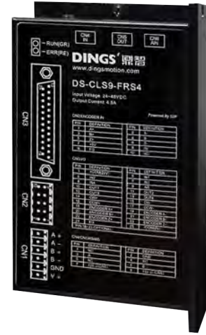
DS-CLS9-FRS4 Stand Alone Closed Loop - Communication Type Driver Apply to Size 6, 8, 11, 14, 17, 23 of Step Motors
