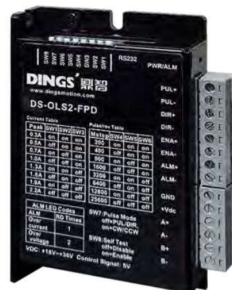
DS-OLS2-FPD Driver Apply to Size 8, 11, 14, 17 of Step Motors
